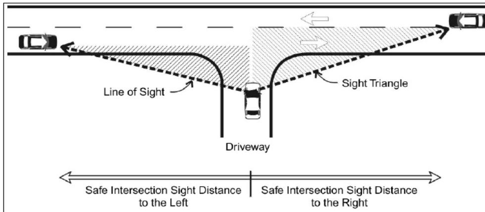
FIGURE 8 – MN/DOT ACCESS MANAGEMENT MANUAL – INTERSECTION SIGHT DISTANCE
