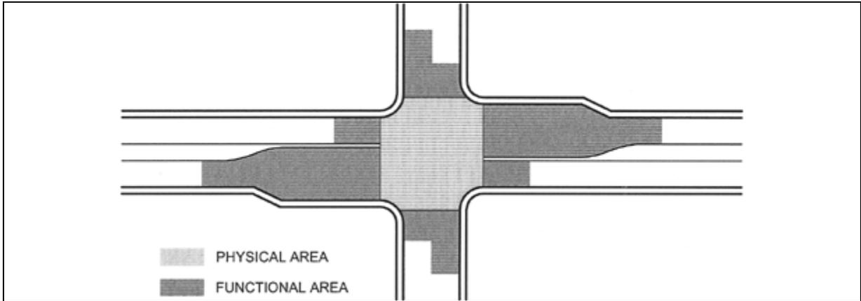
FIGURE 2 - COMPARISON OF PHYSICAL AND FUNCTIONAL AREAS OF AN INTERSECTION
